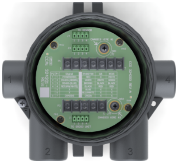
Figure 23 Junction Box Electrical Connections
